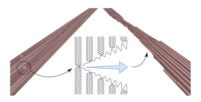
Rice University researchers found that cyclic loading of nanotube fibers leads to strain ratcheting that can eventually lead to the failure of the fiber. Credit: Nitant Gupta and Evgeni Penev / Yakobson Research Group
