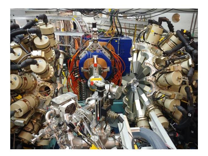
The Argonne Gas-Filled Separator (AGFA) at Argonne National Laboratory's ATLAS facility. The Gammasphere array for HPGe detectors, which is also shown, was not used in this work, but will be a key component of future studies. Credit: Doherty et al.
