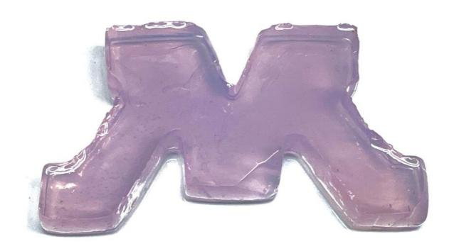
\*This is not jello.\* This block M is composed of engineered bacteria and silica—a material commonly used in plaster—cross-linking together. The purple tint is a protein produced by the bacteria. If the M was damaged, researchers could add nutrients and any cracks would self-heal. Credit: Dr. Sunyoung Kang, Postdoctoral Associate, Schmidt-Dannert Lab.
