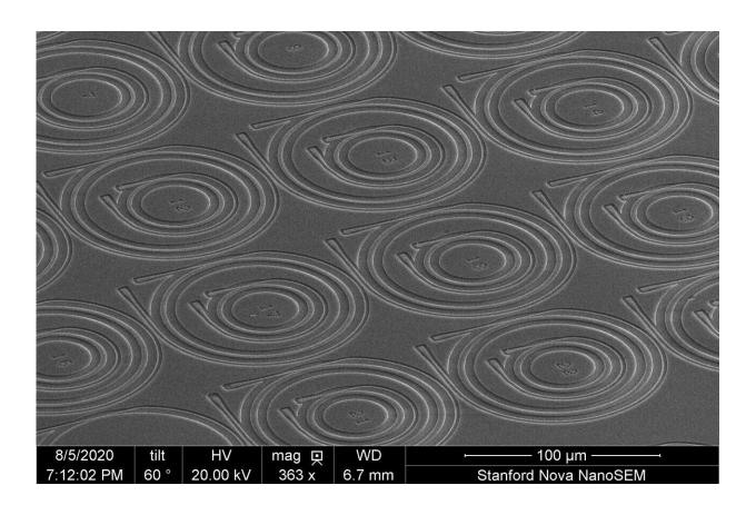
The silicon carbide microrings developed by the Vučković Lab, as seen through a scanning electron microscope at the Stanford Nano Shared Facilities. Credit: Vučković Lab
