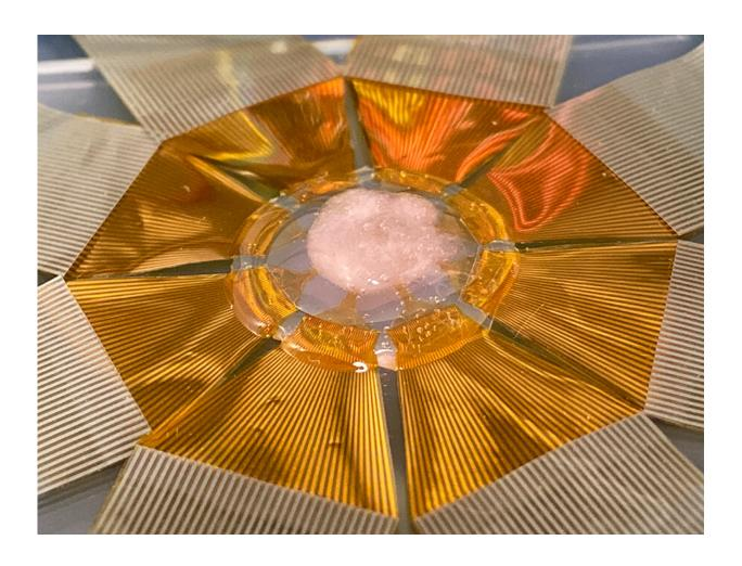
Device with a scaled-up FET sensor array for measuring electrical signals in a 3D cardiac tissue construct. Credit: Yue Gu
