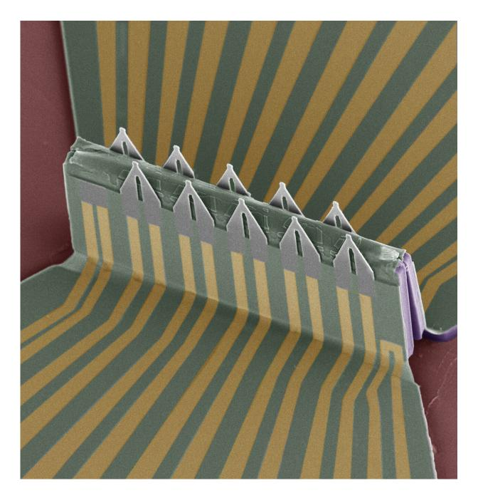
SEM image of the "pop-up" sensors that directly measure speed and movement of electrical signals inside heart cells. Credit: Yue Gu
