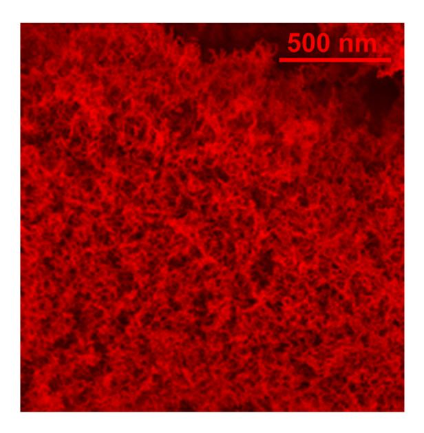
The sponge-like internal structure of the aerogel. Credit: Laboratory for Multifunctional Materials / ETH Zurich
