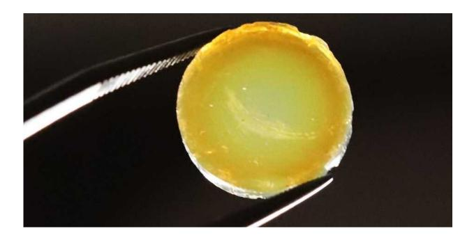
A tablet-shaped aerogel composed of palladium and nitrogen-doped TiO2 nanoparticles. Credit: Markus Niederberger / ETH Zurich
