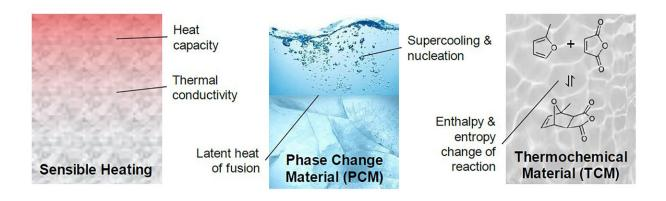
Overview of different thermal energy storage materials and the key properties that require prediction and control for optimal performance over a range of applications. Credit: Ravi Prasher
