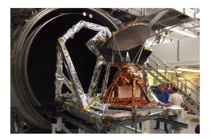
The COWVR instrument during a thermal test in 2015. Credit: NASA/JPL-Caltech
