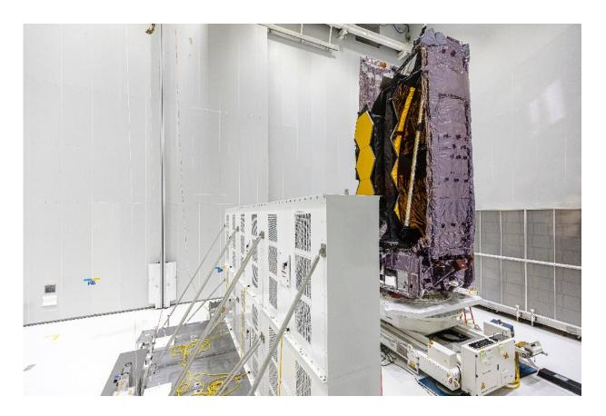
The telescope is so large that it had to be folded to fit into the rocket.
