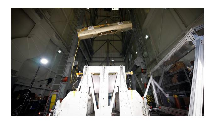
A mock rocket is thrown into the air at NASA's Jet Propulsion Laboratory during tests of a launch system that would fire a rocket off of Mars. The rocket would be part of a multi-mission effort to return Martian samples back to Earth for closer study. Credit: NASA/JPL-Caltech
