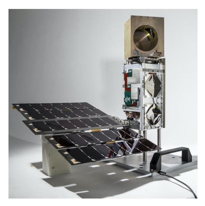
The TROPICS Pathfinder satellite, pictured above, was launched on June 29. The satellite body measures approximately 10 cm X 10 cm X 36 cm and is identical to the six additional satellites that will be launched in the constellation in 2022. The golden cube at the top is the microwave radiometer, which measures the precipitation, temperature, and humidity inside tropical storms. Credit: Blue Canyon Technologies
