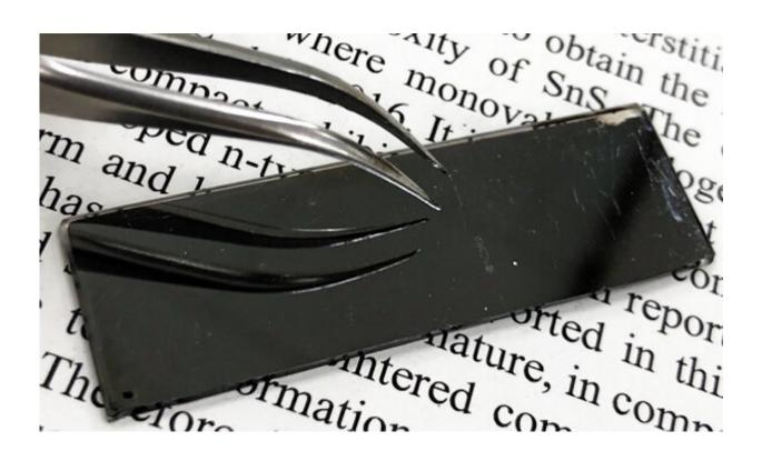
The world's first n-type conductive SnS thin film without containing toxic elements. Credit: Issei Suzuki et al.
