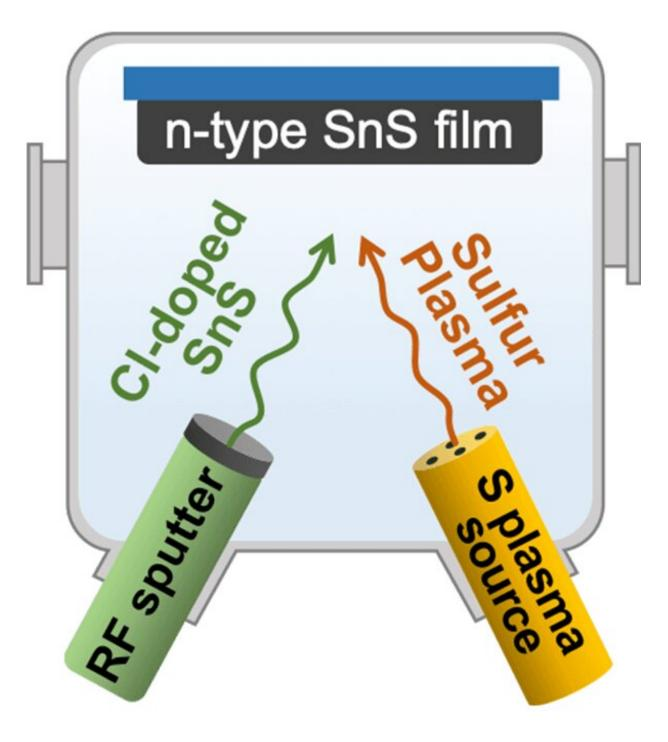
A schematic illustration of the new technique used to fabricate n-type SnS thin films. The n-type conductive SnS thin films were achieved by fabricating thin films of chlorine(Cl)-doped SnS with a supply of sulfur plasma. Credit: Issei Suzuki et al.
