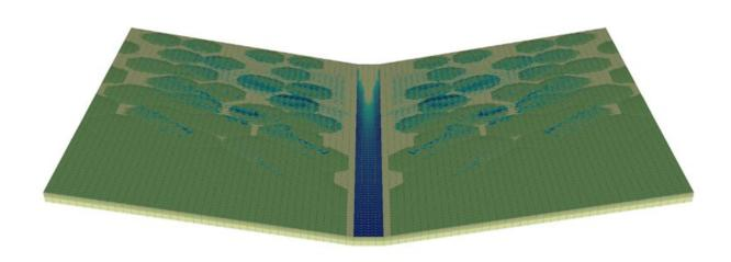
A sample simulation showing a polygonal landscape with variable vegetation cover (green) and surface water (blue) during a rainstorm. The porous, organic-rich soil beneath the vegetation can store a large amount of water, changing the flow of water. Credit: Ethan Coon, Oak Ridge National Laboratory
