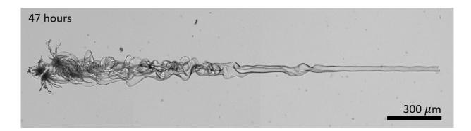
An optical micrograph of a several millimeters long BaCO3-silica nanocomposite. The nanocomposite is grown using a dynamic UV light pattern. By moving the UV light pattern at the correct speed ahead of the growth front, where the building blocks are generated, the researchers can control the growth direction of nanocrystals. It took 47 hours to grow this millimeters-long line of nanocrystals. Credit: Bistervels et al., AMOLF
