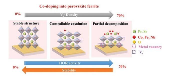
A figure that explains the modulation of the stability and activity of the SOFC anode confirmed by the researchers in this study. As the level of cobalt increases, the hydrogen oxidation reaction (HOR) activity in the anode increases but at the same time, the lattice oxygen bonding increases which heightens the risk of deterioration of the material stability. Credit: POSTECH
