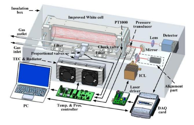
Schematic diagram of the developed dual gas sensor. Credit: Shao Ligang
