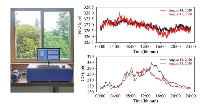
Field deployment photograph and time series of N2O and CO measured concentration using the developed sensor from outdoor air during 48 h on August 14-15, 2020. Credit: Shao Ligang
