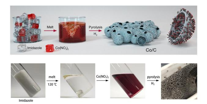
Schematic illustration for the synthesis of Co/C and the photograph of the synthesis steps. Credit: Science China Press
