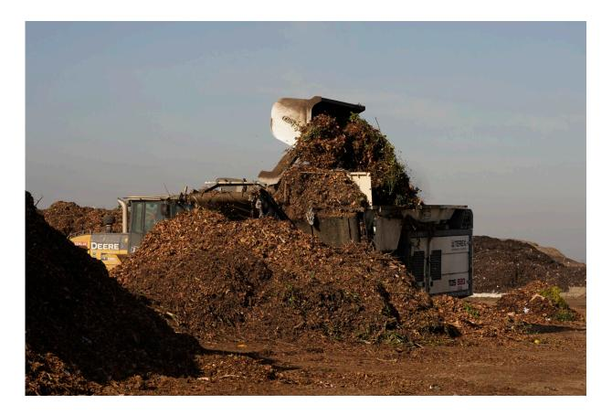
Garden waste is dumped into a grinding machine with other compostable items at the Anaerobic Composter Facility at the Yolo County Central Landfill in Woodland, Calif., Tuesday, Nov. 30, 2021. In January 2022, new rules take effect in California requiring cities and counties to collect food waste alongside green waste for composting. It's designed to reduce greenhouse gas emissions from landfills. Credit: AP Photo/Rich Pedroncelli
