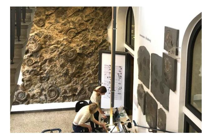
Experimental setup for the drop height of water drops of 430 centimeters in the stairwell in the paleontological collection (Sigwartstr. 10, Tübing-en). At the upper end of the tube the water drops were sent on their journey, at the bottom near the floating fern leaves the high-speed camera is set up. Credit: University of Tübingen
