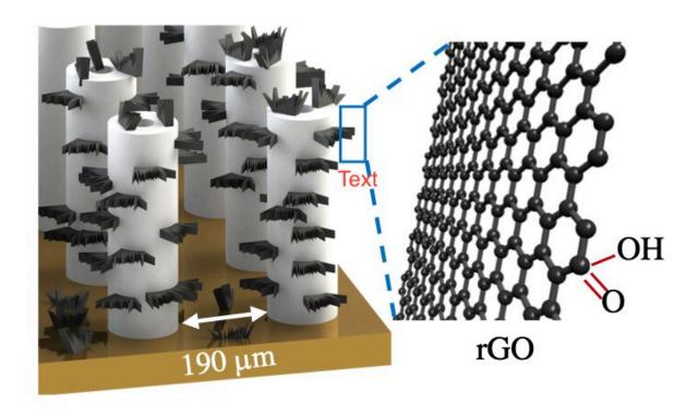
Leveraging additive manufacturing and nanotechnology, Carnegie Mellon University researchers develop a sensor to detect levels of the neurotransmitter dopamine down to femtomolar concentrations. Credit: Advanced Manufacturing and Materials Laboratory, Carnegie Mellon University
