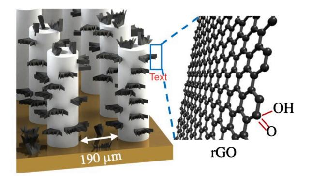
Leveraging additive manufacturing and nanotechnology, Carnegie Mellon University researchers develop a sensor to detect levels of the neurotransmitter dopamine down to femtomolar concentrations. Credit: Advanced Manufacturing and Materials Laboratory, Carnegie Mellon University
