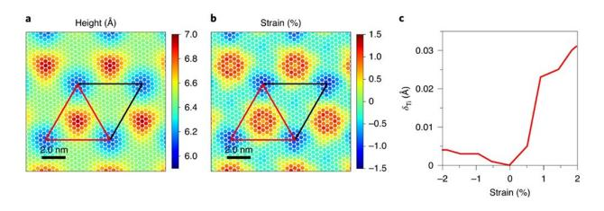
Fig. 4 Relative height and strain field of the heterostructures. Credit: IoP
