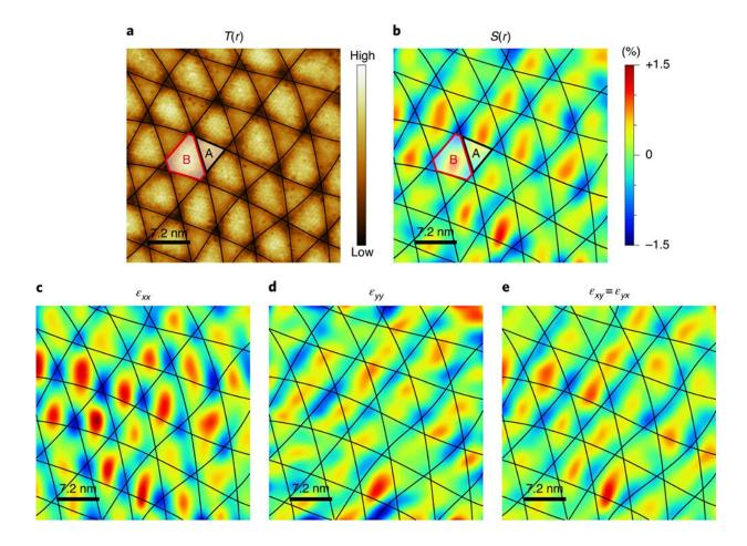
Fig. 3 Symmetric strain map. Credit: NJU
