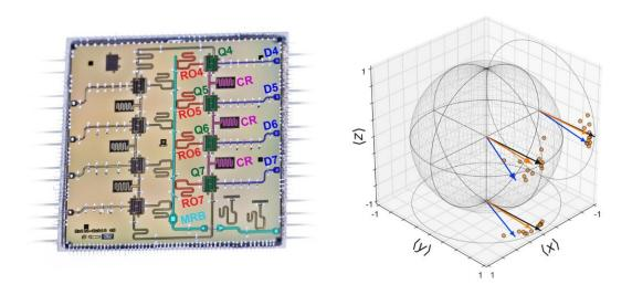
Experimental demonstration of error mitigation through randomized compiling. Left: Eight-qubit superconducting quantum processor. Right: Quantum state tomography of a single qubit with (orange) and without (blue) randomized compiling compared to the ideal (black) state. Credit: Akel Hashim/Berkeley Lab
