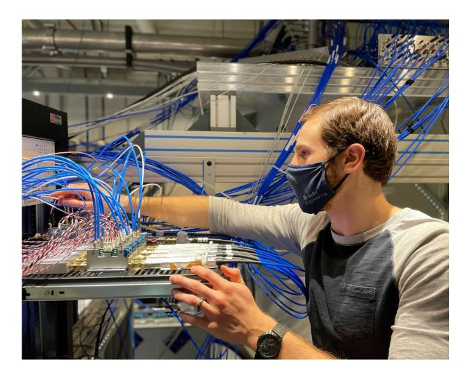
AQT researcher Akel Hashim working on room temperature electronic control systems for superconducting quantum processors. Credit: Christian Jünger/Berkeley Lab
