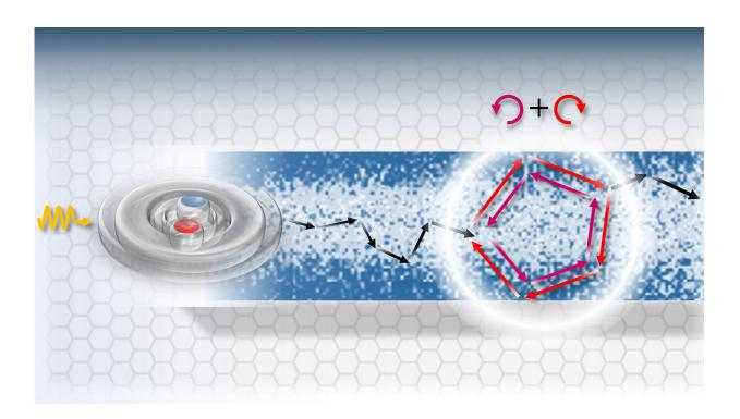
The figure shows a schematic illustration of an exciton excited by a light pulse and moving along an atomically-thin layer. The exciton scatters and randomly changes its direction. In addition, a quantum mechanical interference effect can occur with the exciton propagating through a close loop in both directions at the same time. Credit: Alexey Chernikov
