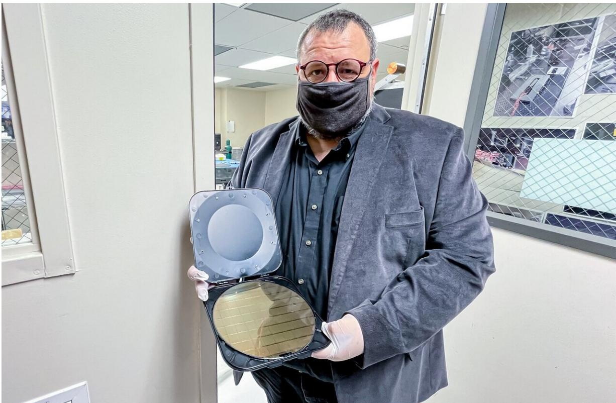
SLAC's Angelo Dragone shows a silicon wafer containing about 50 ePixHR core application-specific integrated circuits, or ASICs. They are the first generation of high-rate readout chips for detectors at the lab's next-generation X-ray laser, LCLS-II. Credit: Jacqueline Ramseyer Orrell/SLAC National Accelerator Laboratory
