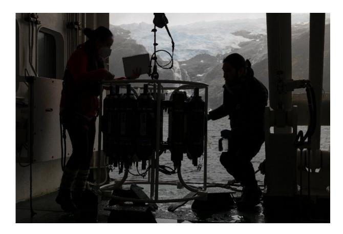
The expedition stopped at 14 places, each time taking water samples at different levels up to a depth of 200 meters using a piece of equipment called a rosette.
