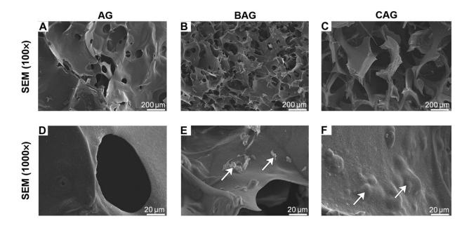
Cross-sectional images of different hydrogels using SEM analysis. (A to C) SEM images of AG, BAG, and CAG. (D to F) Magnified images of AG, BAG, and CAG. White arrows in (E) and (F) indicate the BG and NBG particles on the hydrogel surface. Credit: Science Advances, 10.1126/sciadv.abj7857
