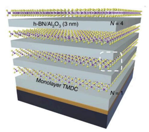
So-called "two-dimensional" materials have unique electrical and photonic properties, but their ultra-thin form factors present practical challenges when incorporated into devices. Penn Engineering researchers have now demonstrated a method for making large-area "superlattices" — layered structures containing 2D lattices of sulfur and tungsten — that can achieve light-matter coupling. Credit: University of Pennsylvania
