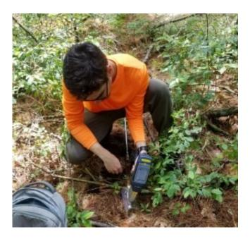
Researcher Mark Higgins testing soil with a probe that is used to collect soil samples at depth. Credit: Mark Higgins
