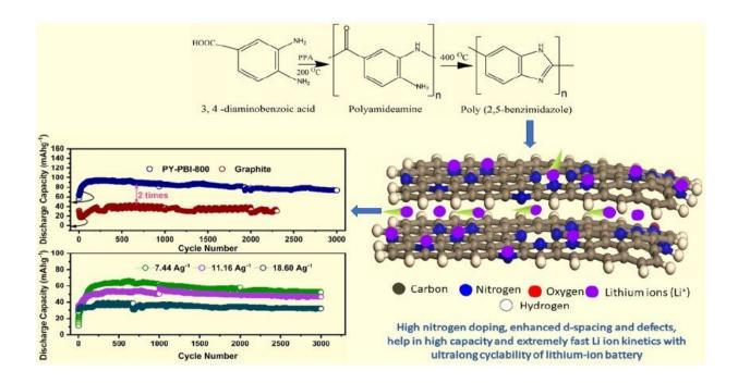
Figure 2. A highly promising anode material for lithium-ion batteries. Some of the key features that makes the proposed material ideal for fast charging are its high nitrogen content and enhanced interlayer spacing, which collectively allow for faster lithium ion kinetics both across and between layers. To top this off, the proposed anode material is very stable and retains most of its original capacity even after thousands of cycles. Credit: Noriyoshi Matsumi from JAIST
