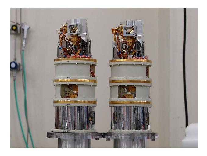
Extremely weak signals from space are collected by the ALMA antennas and focussed onto receivers, like these two shown here, which transform the faint radiation into an electrical signal. The upgraded Band 6v2 receivers will increase both the quality and quantity of science that ALMA can achieve in the band, allowing for more accurate and efficient science. Credit: ESO
