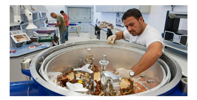
Patricio Escarate, a cryogenics and vacuum technician at the Atacama Large Millimeter/submillimeter Array (ALMA) works on a front end, or chilled cooler that hold the cutting edge receivers for each ALMA antenna. Credit: M. Alexander, ESO
