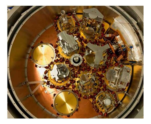
Behind the dish of each ALMA antenna sits one of these Front Ends, the chilled coolers that hold the suite of cutting-edge receivers. Each receiver was hand-crafted in one of three different laboratories around the world. They were brought together to be assembled into this cryogenic unit and shipped to Chile for installation inside each of ALMA's 66 antennas. Credit: P. Carrillo, ALMA (ESO/NAOJ/NRAO)
