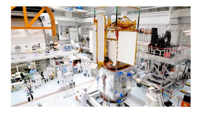
Engineers integrate separate parts of the SWOT satellite into one in a clean room facility in Cannes, France. Credit: Thales Alenia Space
