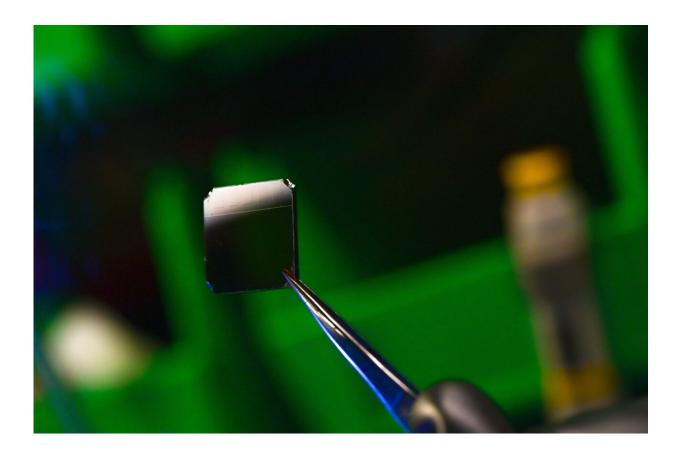
A two-dimensional coat of a perovskite compound is the basis for an efficient solar cell that might stand up to environmental wear and tear, unlike earlier perovskites. Engineers at Rice University raised the photovoltaic efficiency of 2D perovskites by up to 18%. Credit: Jeff Fitlow/Rice University
