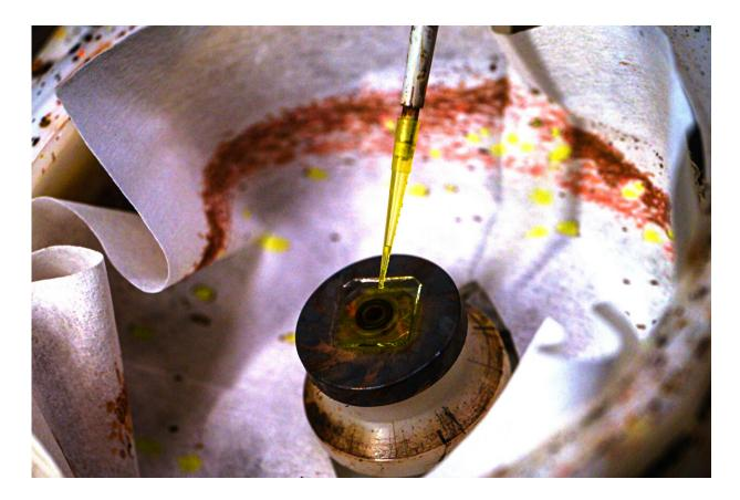
Rice University graduate student Siraj Sidhik prepares to spin-coat a substrate with a compound that solidifies into a 2D perovskite. Rice engineers have found the perovskite shows promise for efficient, robust solar cells. Credit: Jeff Fitlow/Rice University
