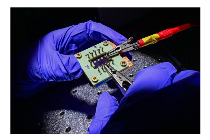
Rice University graduate student Wenbin Li prepares a 2D perovskite solar cell for testing in a solar simulator. Rice engineers boosted the efficiency of cells made of two-dimensional perovskites while retaining their toughness. Credit: Jeff Fitlow/Rice University
