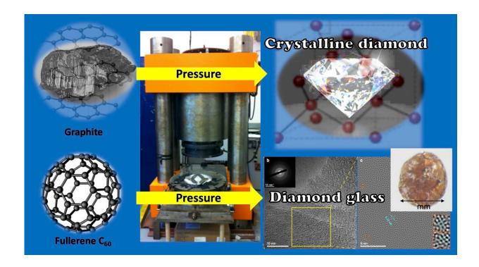
Researchers use multi-anvil press to turn fullerene C60 into diamond glass, similar to the process of converting graphite to diamond in high-pressure apparatus. Credit: Yingwei Fei.
