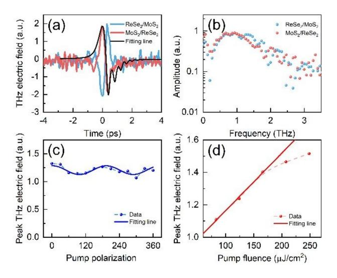
Time-resolved and frequency-resolved THz photoconductivity excited with 800 nm pump pulses in  $ReSe_2$  monolayer and  $MoS_2$ - $ReSe_2$  heterostructures. Credit: Yang Jin
