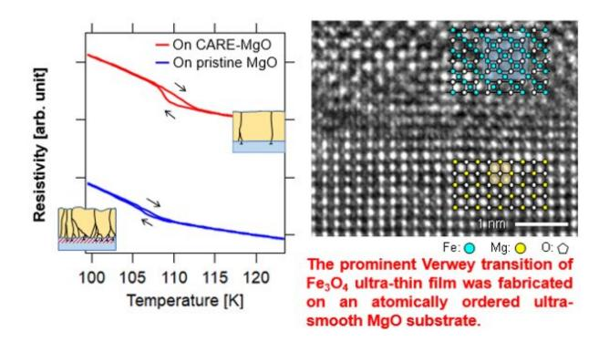
Fig.3 Transition properties of a high-quality magnetite ultrathin film. A clear change in resistivity was observed. Credit: Ai I. Osaka et al.
