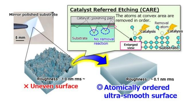
Fig.2 A schematic of our original polishing technique, CARE. Selective removal of atoms from the convex hull leads to an atomically flat surface. Credit: Ai I. Osaka et al.
