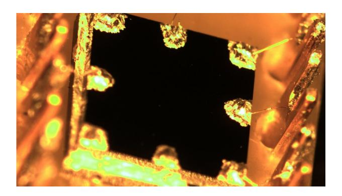
Princeton researchers created the world's purest sample of gallium arsenide, a semiconductor used in specialized systems such as satellites. This photo shows the sample wired inside an experimental setup that looked at electrons in a two-dimensional plane. The sample's purity revealed bizarre effects under relatively weak magnetic field, behavior that has no established theoretical framework. Credit: Princeton University
