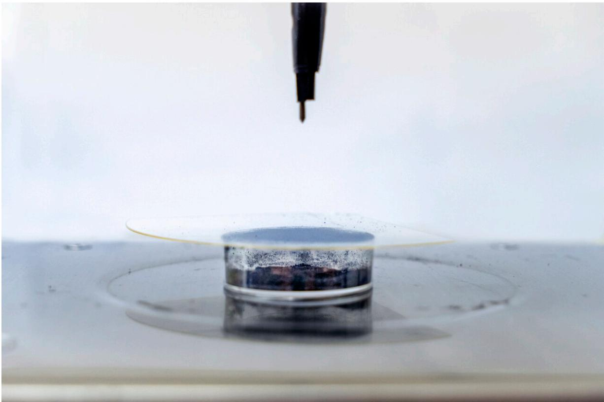
Corona-Enabled Electrostatic Printing prints electronic skin, or “e-skin,” by using corona discharge to create a strong electric field between binder-free functional powders, such as graphene, and flexible, non-conductive surfaces, such as medical tape. The electrostatic force enables a multitude of e-skin sensors to be printed within sub-seconds, compared to the 20 minutes it takes with polymer binders, and doesn't require heat. Credit: University of South
