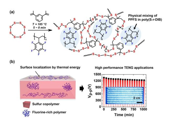
Toxic gas-free synthesis of sulfur copolymer and fluorine-rich polymer blends.(a) schematic of synthesis of the polymer blend through inverse vulcanization.(b) Migrated fluorine-rich polymer to the surface of polymer blend film by thermal energy, achieving high triboelectric performance. Credit: Inha University
