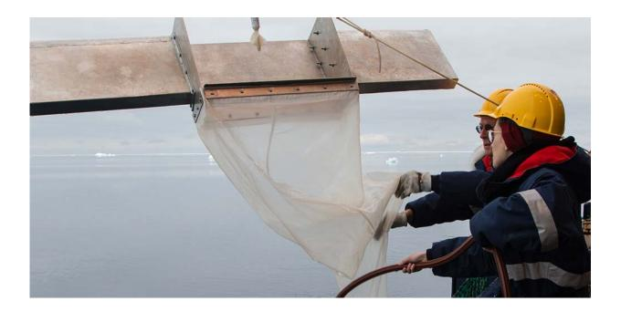
The plankton net used to sample the water surface is rinsed off before sampling to remove any particles that may have adhered beforehand. Credit: University of Basel, Patricia Holm
