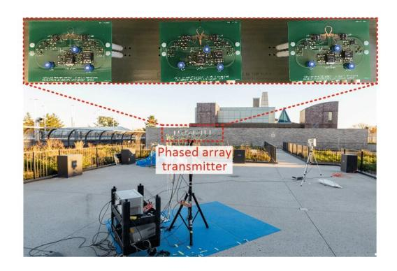
Princeton researchers have developed a new type of phased array antenna based on large-area electronics technology, which could enable many uses of emerging 5G and 6G wireless networks. The researchers tested the system on the roof of Princeton's Andlinger Center for Energy and the Environment. Credit: Can Wu
