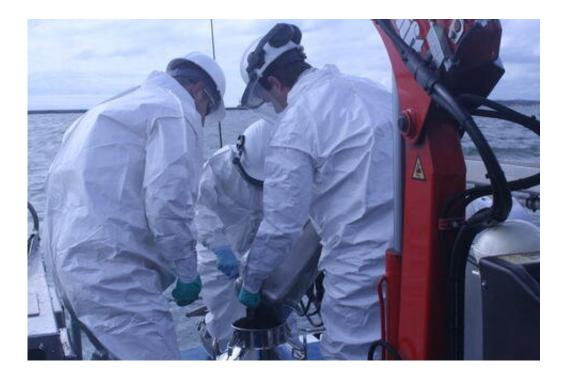
NIST researchers collected sediment material from three different sites in Milwaukee Bay. The sediment was put in stainless steel milk cans for storage before being transported to Hollings Marine Laboratory for sample analysis. Credit: M. Ellisor/NIST
