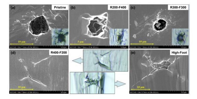
Nanosecond laser-induced damage morphologies of DKDP crystal after subnanosecond laser conditioning with different temporal shapes. Credit: SIOM
