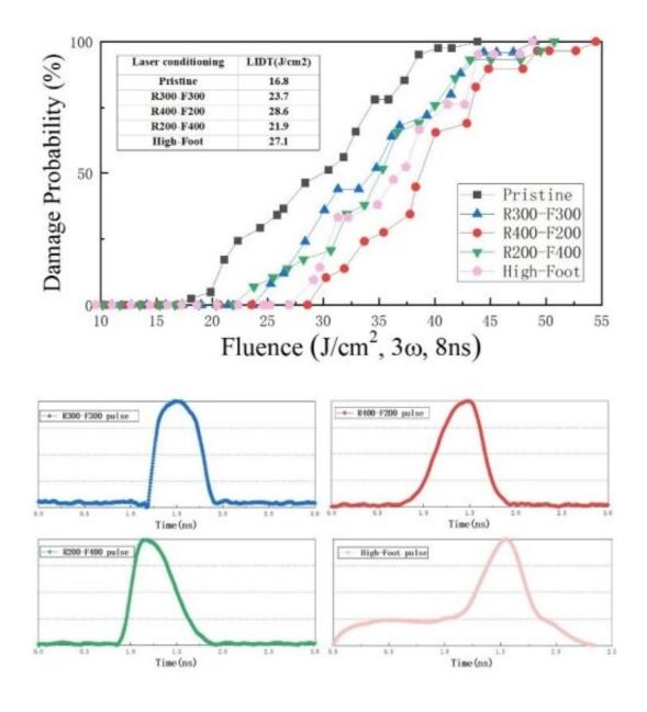
R-on-1 laser-induced damage thresholds of DKDP crystals before and after laser conditioning with different temporal shapes. Credit: SIOM
