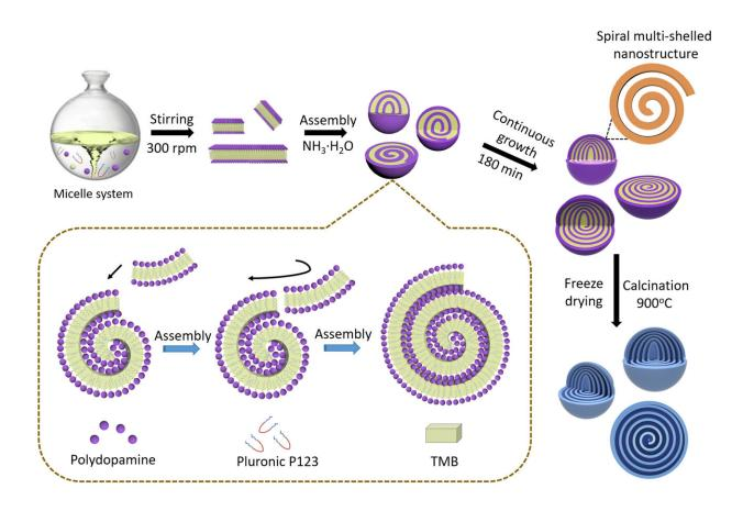
Schematic representation of the formation process of the spiral MCNs. First, the lamellar micelle system was formed by stirring the reactant at 300 rpm. Then, the lamellar micelles were dynamically assembled into the mesostructured PDA nanospheres under the guidance of the shearing flow. Last, carbonization of the freeze-dried PDA nanospheres in N2 atmosphere could lead to the formation of spiral MCNs with interesting chiral architecture. Credit: Science Advances, doi:
