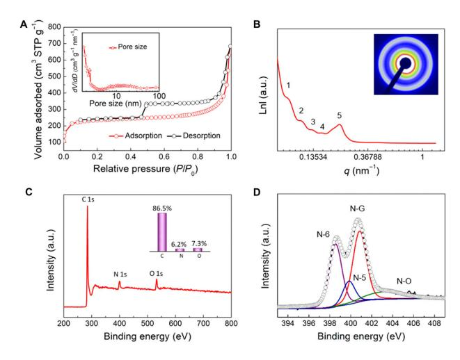
Physicochemical characterization of the spiral MCNs. (A) N2 sorption isotherms, (B) SAXS pattern, (C) XPS survey, and (D) high-resolution N 1s XPS spectrum of the mesoporous MCNs with unique chiral architecture prepared by the lamellar micelle spiral self-assembly strategy. Insets in (A) to (C) are the corresponding pore size distribution, two-dimensional SAXS image, and element weight percentages, respectively. a.u., arbitrary units. Credit: Science Advances, doi: 10.1126/sciadv.abi7403
