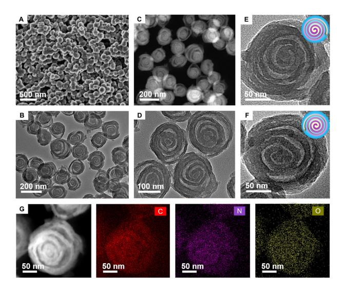
Microstructure characterization of the spiral MCNs. (A) FESEM image, (B and D) TEM image, (E and F) magnified TEM images, and (C and G) scanning TEM and energy-dispersive x-ray element mapping images of the mesoporous MCNs with unique chiral architecture prepared by the lamellar micelle spiral self-assembly strategy. Credit: Science Advances, doi: 10.1126/sciadv.abi7403
