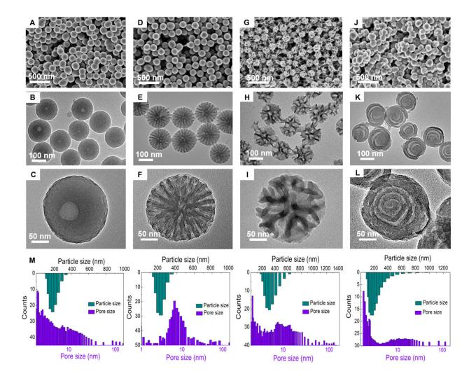
The controllability and versatility of the synthetic method. FESEM and TEM images of the mesoporous carbon nanospheres prepared by adjusting the interfacial curvature of micelles through using different Pluronic triblock copolymers: (A to C) F108, (D to F) F127, (G to I) P105, and (J to L) P123. (M) The corresponding distribution histograms of the particle diameters and pore sizes. Credit: Science Advances, doi: 10.1126/sciadv.abi7403
