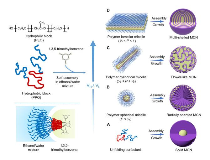
Schematic illustration of the formation mechanism for the mesoporous carbon nanospheres with diverse architectures. A series of mesoporous carbon
