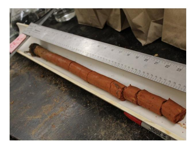
Scientists collect cores of soil at various depths. Shown, a soil core of about two feet is measured and sectioned into respective depths for soil testing. Several chemical, physical and biological tests are better or worse for different kinds of soil. Credit: Anjan Bhatta
