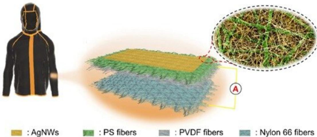
Made of electrospun polyvinylidene fluoride (PVDF) and nylon, silver nanowires (AgNWs) and polystyrene (PS), the new all-fibrous composite nanogenerator (AF-TENG) can be easily incorporated into clothing, allowing it to power small electronics through everyday movements. Credit: Elsevier
