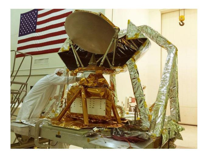
The COWVR instrument (center, wrapped in gold foil) in JPL's Environmental Test Laboratory during vibration testing. Credit: NASA / JPL-Caltech
