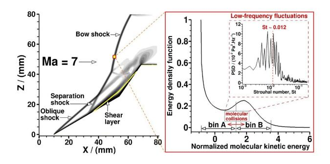
Left: shock-wave/boundary-layer interactions in a Mach 7 flow over a oublewedge configuration. Right: a bimodal energy distribution function of particles in the bow shock. Molecular collisions between the low energy bin A and high energy bin B cause low-frequency fluctuations having Strouhal number on the order of 0.012. Credit: University of Illinois Dept. of Aerospace Engineering
