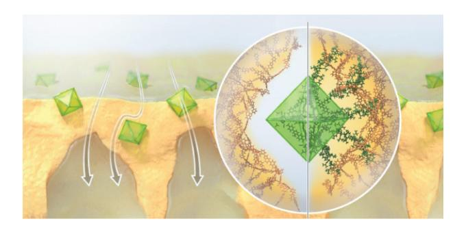
KAUST chemical engineers have developed a new separation technology using mixed-matrix membranes containing metal-organic framework fillers. The new technology consumes up to 90 percent less energy than conventional separation techniques. Credit: Xavier Pita.
