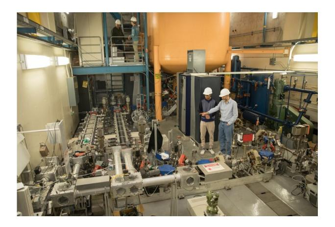
Mark Sherwin (bottom right) explains the inner workings of the free-electron laser. The large yellow tank accelerates electrons, which are guided along the beam line and into the "wigglers" at the far left. Credit: UC Santa Barbara
