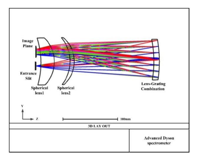
Optical system and prototype for advanced Dyson spectrometer. Credit: Wu Su
